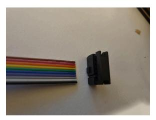
10. Insert the cable and crush the connector onto the wires.
